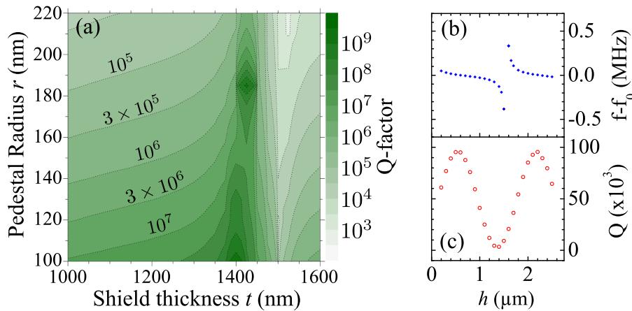
FIG. 3.  $Q$  optimization of the geometry presented in Fig. 2(a). (a) Contour color map in log scale of the calculated  $Q$ -factor of a shielded disk resonator as a function of shield thickness and pedestal radius for  $h = 550$  nm. (b) Radial breathing mode frequency and  $Q$ -factor as a function of the lower pedestal's height  $h$ , with  $(t; r) = (1000; 180)$  nm. Frequency scale is offset by  $f_0 = 1.38$  GHz for clarity.
